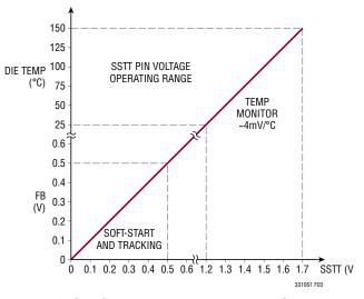
Figure 3. Soft-Start and Temperature Monitor Operation
