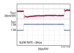
2MHz, 1.0V, Forced Continuous 1.5A DC to 7.5A Step Load 6A/µs Transient, <3% Total Variation
