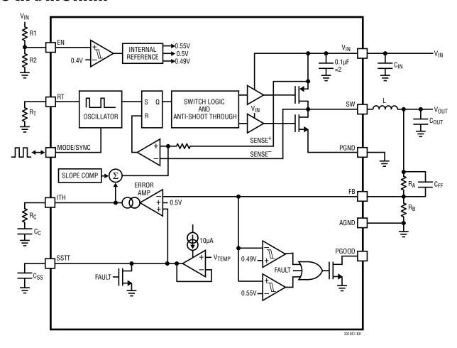
Note: On the LTC3310S-1 the  $R_{\mbox{\scriptsize A}}$  and  $R_{\mbox{\scriptsize B}}$  resistors are internal.
