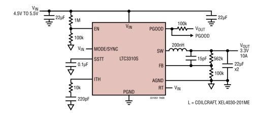
High Efficiency, 2MHz, 0.5V, 10A, Pulse Skip, Low Part Count
