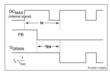
Figure 10. Output Enable Timing.
