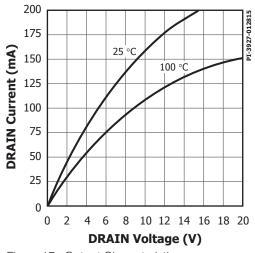
Figure 17. Output Characteristics.
