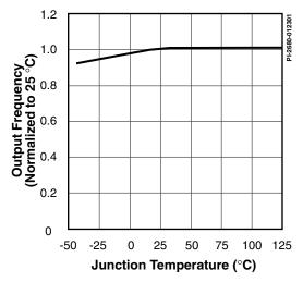
Figure 13. Frequency vs. Temperature.
