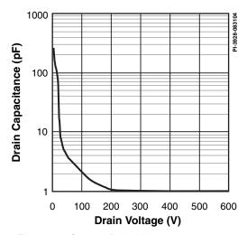
Figure 18.  $C_{\rm oss}$  vs. Drain Voltage.
