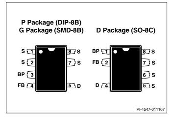
Figure 3. Pin Configuration.
