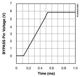
Figure 16. BYPASS Pin Startup Waveform.
