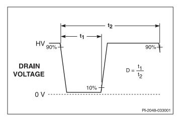
Figure 9. Duty Cycle Measurement.
