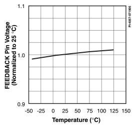
Figure 15. FEEDBACK Pin Voltage vs. Temperature.
