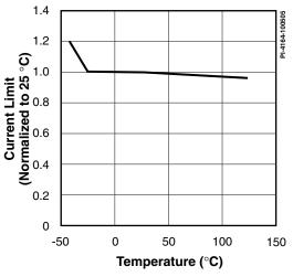
Figure 14. Current Limit vs. Temperature.
