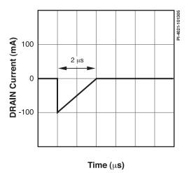
Figure 11. Peak Negative Pulsed DRAIN Current Waveform.
