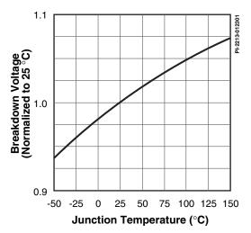
Figure 12. Breakdown vs. Temperature.
