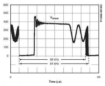
Figure 4. Frequency Jitter at fosc
