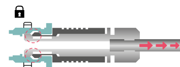
Secure locking when cable pulled
