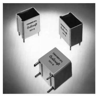
These low cost Coilcraft current sensing transformers are designed for use up to 1 MHz. They incorporate the current and sense windings in one small, encapsulated package requiring minimum board space.
