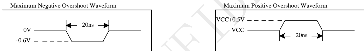
Figure 5-1 Maximum Overshoot Waveform
