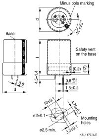
Snap-in capacitors are also available with 3 terminals (length (4.5 – 1.4) mm). PET insulation cap is positioned under the insulation sleeve.
