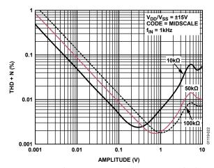
Figure 22. Total Harmonic Distortion Plus Noise vs. Amplitude
