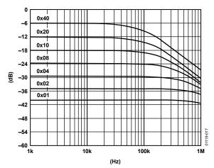
Figure 17. 50 k $\Omega$  Gain vs. Frequency vs. Code
