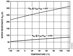
Figure 13. Wiper Contact Resistance vs. Temperature
