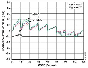
Figure 8. Potentiometer Divider Nonlinearity Error vs. Code
