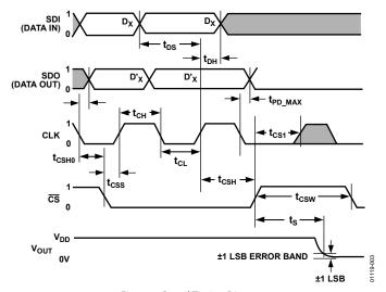
Figure 3. Detail Timing Diagram
