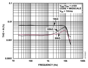
Figure 21. Total Harmonic Distortion Plus Noise vs. Frequency
