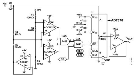
Figure 35. Audio Volume Control with Zipper Noise Reduction
