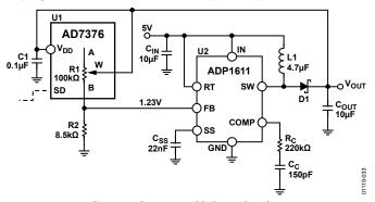
Figure 33. Programmable Power Supply
