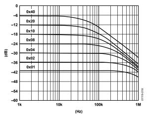
Figure 18. 100 k $\Omega$  Gain vs. Frequency vs. Code
