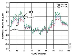
Figure 6. Resistance Step Position Nonlinearity Error vs. Code
