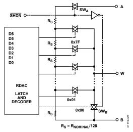
Figure 25. AD7376 Equivalent RDAC Circuit
