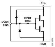
Figure 29. Equivalent ESD Protection Circuit
