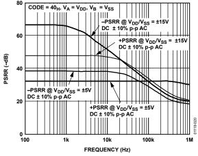
Figure 20. Power Supply Rejection vs. Frequency
