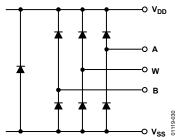
Figure 30. Equivalent ESD Protection Analog Pins
