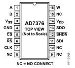
Figure 5. 16-Lead SOIC\_W Pin Configuration
