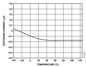
Figure 11. Shutdown Current vs. Temperature
