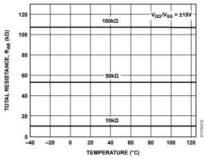
Figure 12. Total Resistance vs. Temperature
