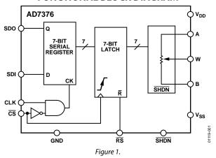
The AD7376 features sleep-mode programmability in shutdown that can be used to program the preset before device activation, thus providing an alternative to costly EEPROM solutions.
