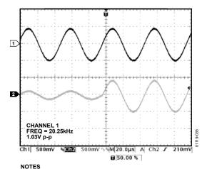
THE LOWER TRACE SHOWS THAT THE VOLUME LEVEL CHANGES FROM QUARTER SCALE TO FULL SCALE, WITH THE CHANGE OCCURRING NEAR THE ZERO-CROSSING WINDOW.
