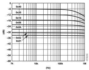
Figure 16. 10 k $\Omega$  Gain vs. Frequency vs. Code
