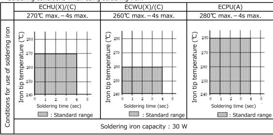
\* Soldering conditions when using soldering iron.
